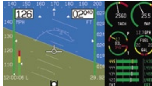
Engine monitor data acquired from Dynon's EMS system
